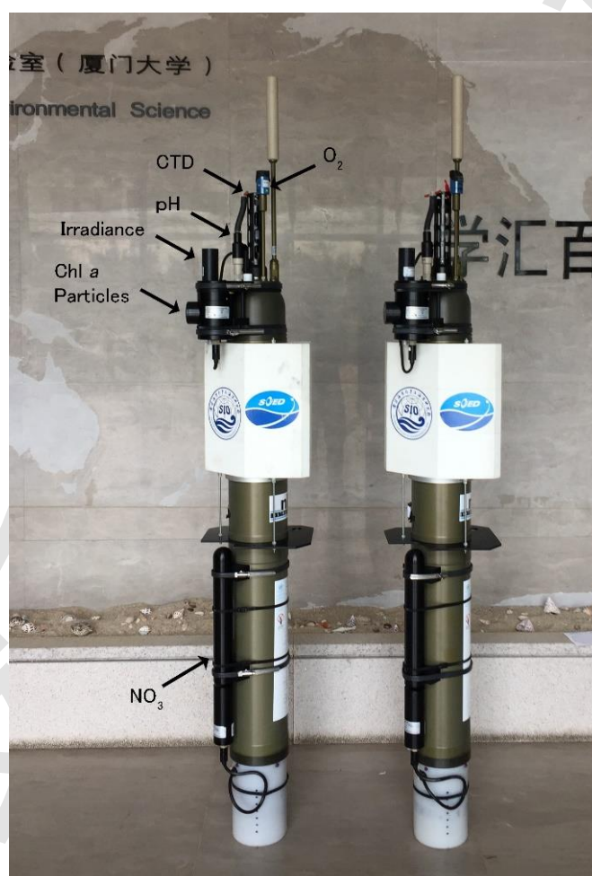
208 209 Fig. 4 BGC Argo floats equipped with CTD and six BGC sensors (oxygen, nitrate, pH, chlorophyll a , 210 suspended particles and downwelling irradiance) (photo courtesy of Xiaogang Xing, Second Institute 211 of Oceanography, Ministry of Natural Resources, China.). 212
