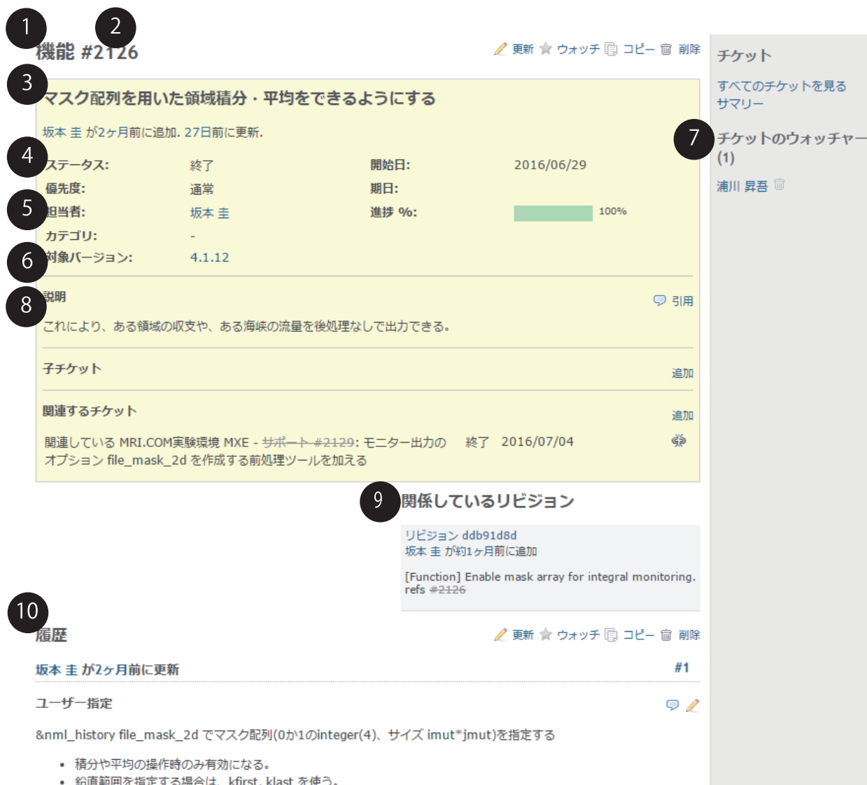
Fig. 4. A Redmine ticket in Japanese made for MRI.COM. The items indicated by circled numbers are as follows: (1) classification (tracker), (2) serial number, (3) title, (4) status, (5) person in charge, (6) release version, (7) reviewer, (8) note, (9) git commit and (10) comments.
