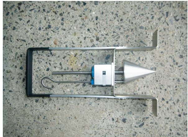
Fig. 2. Penetrometer for Soft Soil.
