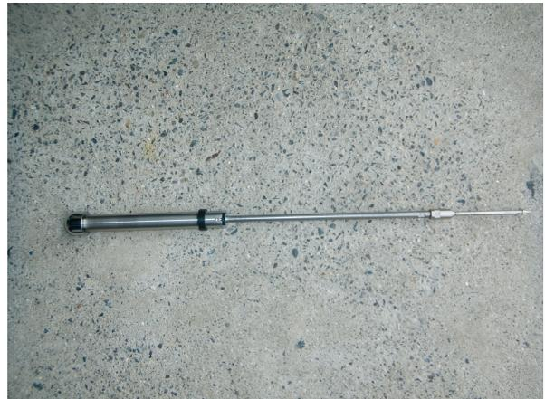
Fig. 1. Device for measuring penetration resistance with corn and spring.
