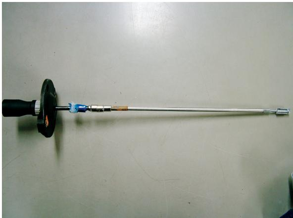
Fig. 5. Torque measurement tool for bolting with vane.
