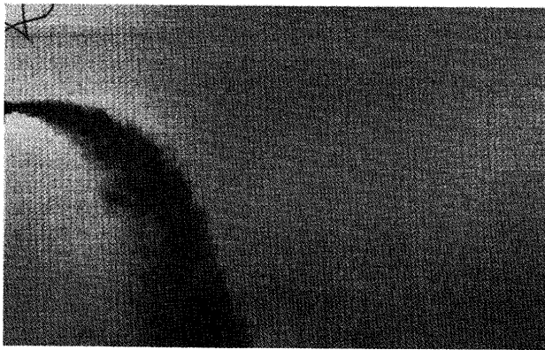
Fig. 9. Visualization of buoyant jet at the conditions of Fr = 6 and Re = 4,000 .
