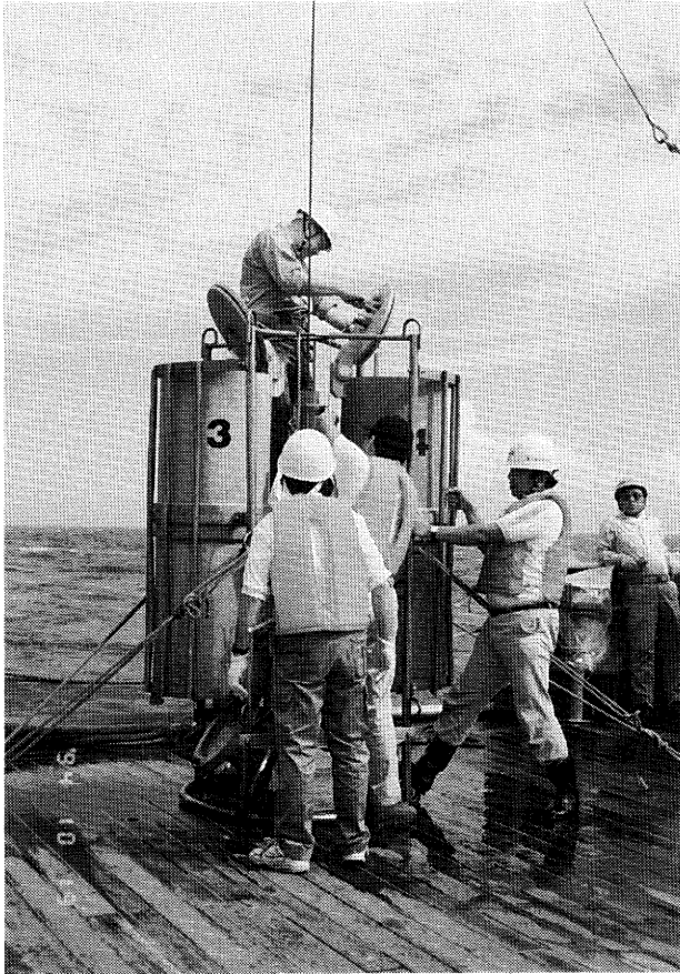
Fig. 4. A photograph of the large-volume (250 L) water sampling system developed by Horibe and Tsubota (1977).
