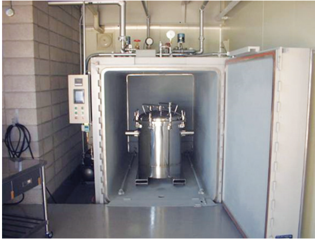
Fig. 1. Photograph showing a giant autoclave and stainless-steel reaction chamber—seawater is autoclaved twice at 120°C for 2 h.
