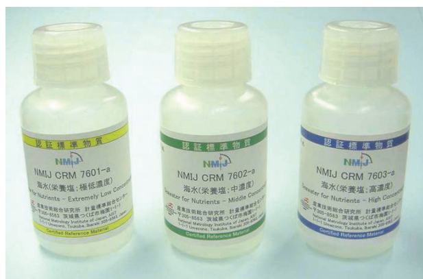
Fig. 5. Photograph of NMIJ CRMs—left: NMIJ CRM 7601-a (extremely low), center: NMIJ 7602-a (middle), right: NMIJ 7603-a (high)
