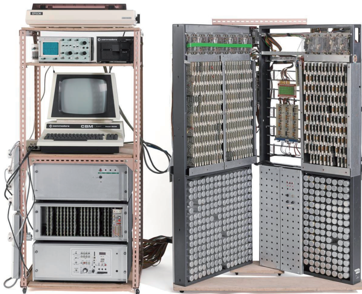
Photo 3. Analog computer developed by Dr. Shizuo Ishiguro since 1977. (a) Main computation cabinet around 1980 at IOS taken from different angles. The dimension of the cabinet is 169 \times 67 \times 64 cm. The base size is 67 \times 105 cm. These photos are cited after Ishiguro (1980) by courtesy of University of Southampton. (b) “Electronic storm surge modelling machine” exhibiting at Science Museum in London. The personal computer (Commodore model CBM8032) and the relating digital circuit components are added later. The dimension of the control rack (left part) is 153 \times 60.8 \times 55 cm, and the analog computation rack in the state exhibited (right part) is 147 \times 100 \times 66 cm. This photo is cited after Science Museum (2015) under the Creative Commons Attribution Non Commercial-Share Alike 4.0 License, ©The Board of Trustees of the Science Museum.
